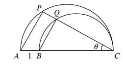
In the figure, AC and BC are diameters of two semi-circles touching each other internally at *C*. *PQC* is a straight line. If AB = 1, then PQ =
