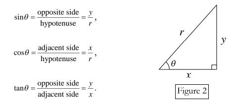
The above definitions are valid for the acute angle  $\theta$ . If  $\theta$  is greater than or equal to 90°, the trigonometric ratios of  $\theta$  are "redefined", as shown in Figure 1 and Table 1.
